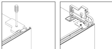
2 Unscrew right top hinge cover, and disconnect connectors of door switch and display.
