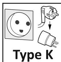
If only a type K socket is available at the point of connection, the device must be connected with a suitable adapter. Only in this way is the device properly grounded.
